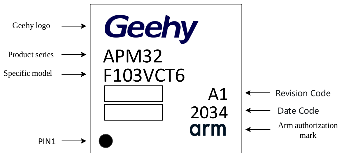
Figure 19LQFP100-100 pins, 14×14mm package identification
